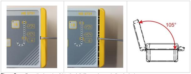
Figure 2. Open the housing lid to the left (figure shows similar device)
