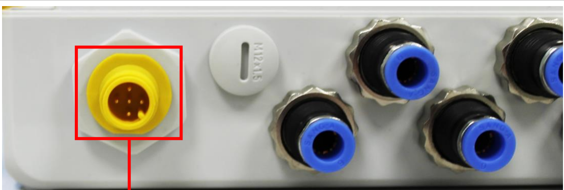
M12 connector plug, 5-pin, A-coded
