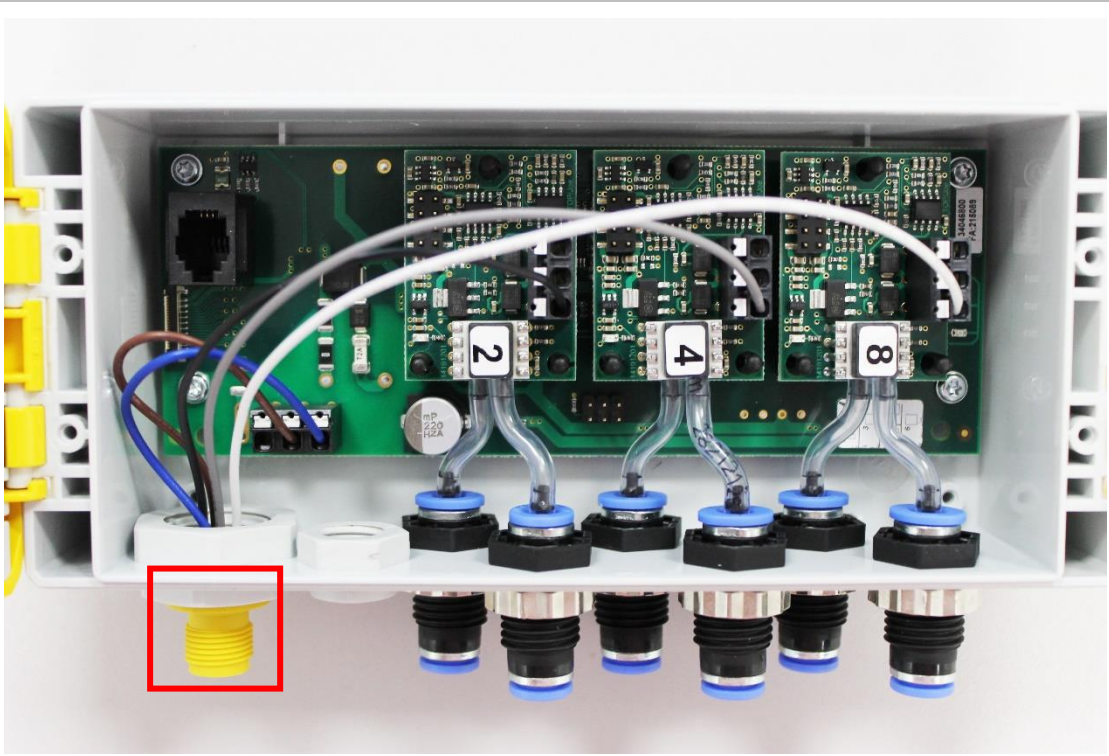
Figure 7 Electrical connection via M12 connector plug
