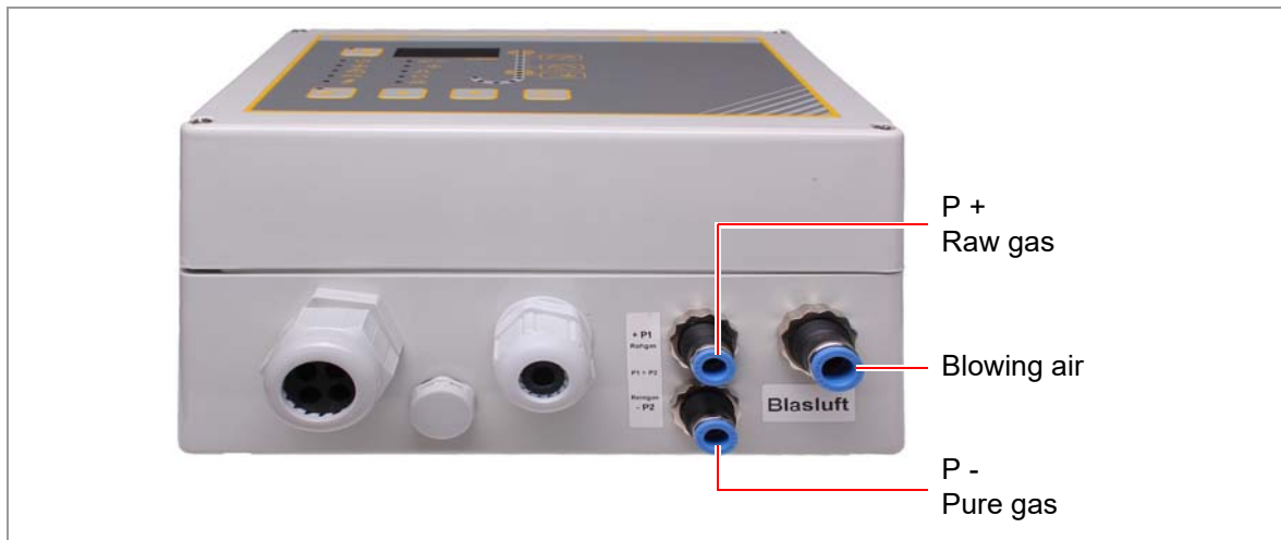
Fig. 7.4: Connection for measuring hose cleaning
