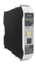
The field bus coupler HE 5813 links the modular process I/O HIMOD system with a Modbus RTU network. The connection to the Modbus RTU is established with a 9-pin D-SUB socket. Up to 62 I/O modules can be connected per bus coupler. The connection of the modules takes place over an internal bus system. Up to 16 modules can be operated directly on the bus coupler, in addition the system can be expanded with an additional power module. In the bus coupler the areas of power supply voltage, field
