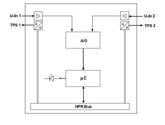
The analogue input module HE 5831 acquires up to two analogue signals from path-, angle- and position sensors and transmits these to the higher-level bus system. The communication with the bus coupler takes place over an asynchronous serial RS485 connection. A short-circuit-proof voltage is provided for the supply of the potentiometric transmitter. Every input has variable MIN- and MAX values, with which an alarm message is reported to the controller managing the process. The module is powered
